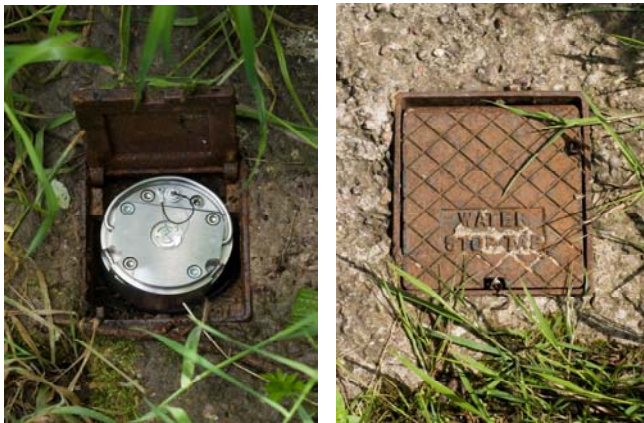
Figure 2. The GasClam® fits in to a standard borehole making it safe and secure on site.
